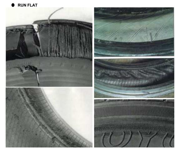
CAUSE: DEFORMATION OF THE CASING CAUSED BY RUNNING TIRE AT EXTREME LOW INFLATION FOR A LONG DISTANCE
