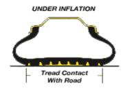
Underinflation causes tire deflection and heat buildup, which increases the risk of failure, it also causes excessive wear on outter tread ribs.
