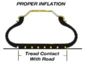
The correct profile for full contact with the road which results in minimum tire performance is shown above.
